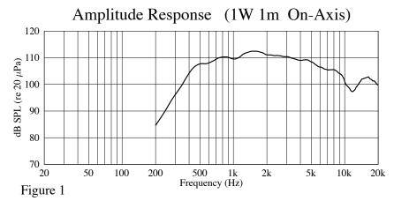
Amplitude response (1W 1m On-Axis) measured on a CH-7 constant directivity horn
