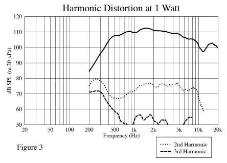
Harmonic distortion at 1 Watt measured on a CH-7 constant directivity horn
