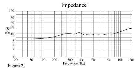
Impedance measured on a Plane-wave terminated tube
