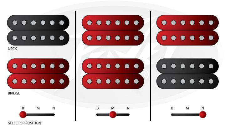
IN MIDDLE POSITION, VOLUME CONTROLS ARE INDEPENDANT SO THAT THE PICKUPS CAN BE BLENDED.
