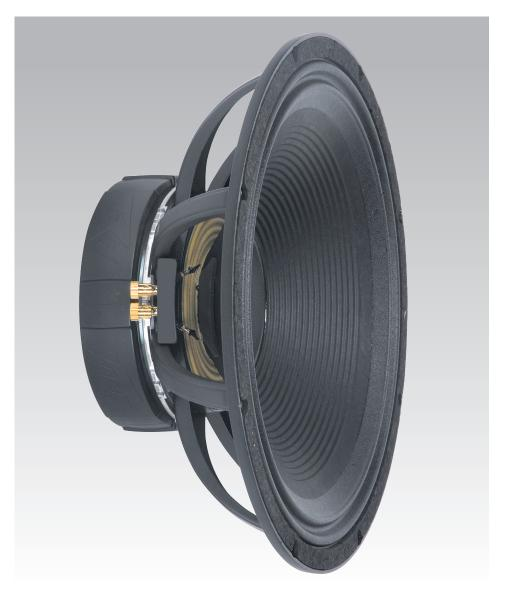
ribbon wire, edge wound and bonded onto an incredibly durable and heat resistant polyamide composite former. With a winding length of 1.150", the long coil has much more surface area to dissipate heat, and its increased length drives the cone to a far higher excursion. The coil is over coated with a tough thermoset
