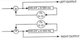
Stereo Multi-tap Echo (Libraries 75-79 and 85-89): Offers up to 680 milliseconds of delay in either of the Left or Right Taps. A single Feedback (FB) is taken from the Tap with the longer delay time. This feedback is also programmable with up to
