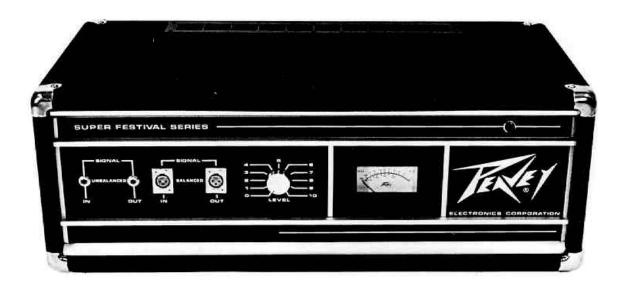
The 800 Booster features our field proven 800 module delivering 400 Watts RMS @ 0.2% THD. The 800 module uses ten high voltage 30 amp power devices mounted on a massive finned aluminum heatsink with the added safety margin of forced air cooling. The thermal tracking circuit as well as the integral thermal cutout are standard features of the 800 Booster.
