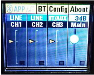
Fig. 3 Main (Master) Channel Gain +3 dB
