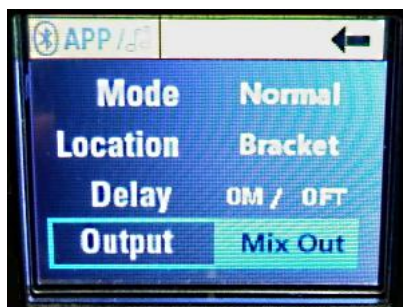
Fig. 30 Output Parameter, Mix Out Selected
