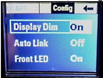
Fig. 48 Display Dim turned On
