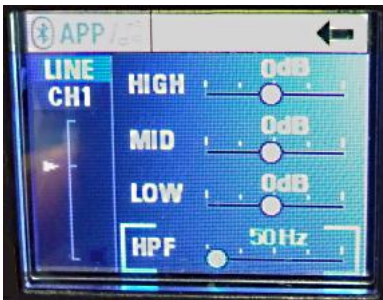
Fig. 15 HPF set to 50 Hz
