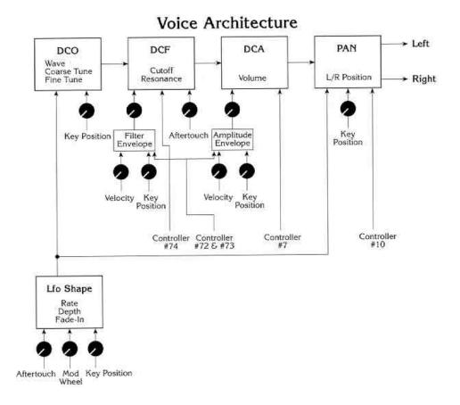
Filter & Amplitude Envelope Structure
