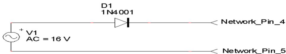
Note that if the combination of cable distance and loading causes a significant voltage drop across the network, a second supply can be connected at the far end of the cable.
